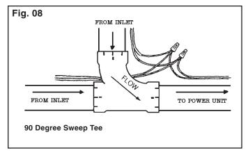
String the low-voltage wire along as you assemble the tubing. Join or splice low-volt wires with wire connectors at each junction or branch in the tubing. To make sure the polarity is right, always attach wires of the same color to each other — typically copper-to-copper and silver-to-silver. Proceed until the tubing system is complete.
