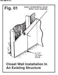
Then, using a length of coat hanger, drill a hole through both walls (Fig. 01). Hold the wire perfectly horizontal so the interior and exterior holes line up with one another. Check for inner wall obstructions by bending a short length of coat hanger wire at a right angle and twirl the right angle piece inside the wall. If there are no obstructions, drill a 2-1/4" (5.7cm) hole horizontally through both walls.
