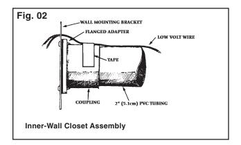
Pass low-voltage wire through the wire guide hole in the inner wall closet assembly (Fig. 02) and tape or cable tie low-voltage wire to this assembly immediately behind the bracket. Attach wires to low-voltage terminals on the back of the inlet valve. Place the inner wall assembly lengthwise through the wall opening and arrange the assembly so the bracket is flush with the inside surface of the wall. Screw the inlet valve to the wall (Fig. 03).
