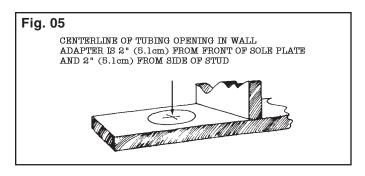
Glue a length of tubing into a stud-mounting bracket assembly. Cut a length of low-voltage wiring, bring approximately 6" (15.24cm) through top wire guide hole in stud bracket assembly and double it back into elbow hole. Tape wire to tubing at assembly elbow and again close to end, and tuck remaining wire into bottom of tubing. Screw plaster guard onto face of assembly (Fig. 06).
