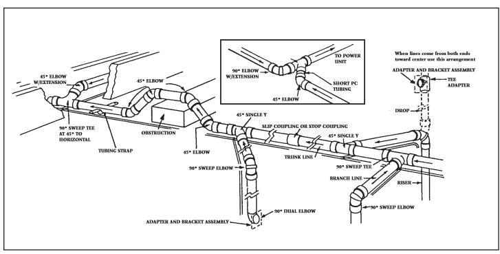
Connect tubing from additional inlet valves to the main trunk line using 90 degree sweep tee elbow fittings. (Fig. 07) and use clamps to hold the sections in place. Be sure to install the sweep tee fittings so the sweep is toward the power unit (Fig. 08). Always run branch lines from the sides or top of the main trunk line, never out of the bottom because this will create a trap for dirt to fall into.
