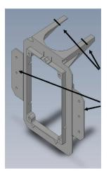
To allow the frame to fit through the valve hole in the sheetrock, cut approximately 3/4" (1.9 cm) off the forks.
