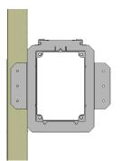
The pipe fitting is designed to slide in the frame to adjust for variations in wall board thickness.
